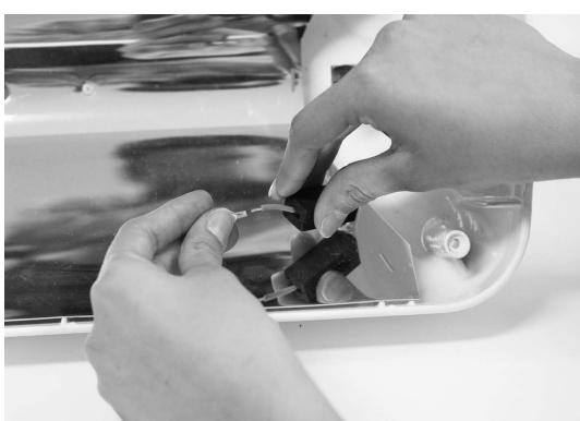
6. RACCORDER LES COSSES (FASTON) MÂLES DU NOUVEAU TUBE À CELLES DES DEUX FILS D'ALIMENTATION, LES RECOUVRIR AVEC LES PROTECTIONS ET REMETTRE LE TUBE DANS SON LOGEMENT DANS LES CLIPS.
