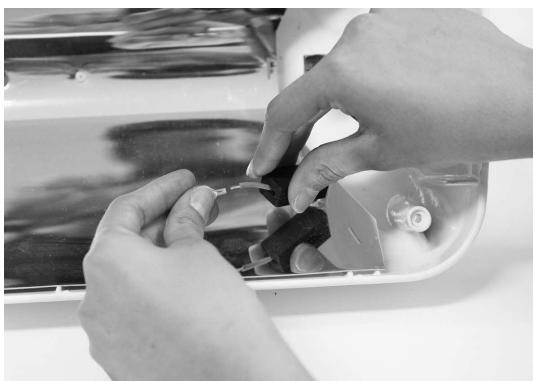
6. CONNECT THE MALE FASTONS OF THE NEW BULB TO THOSE OF THE TWO CORDS. COVER THEM WITH THE HEAT-ELASTIC CAPS AND RE-POSITION THE BULB IN THE SEAT OF THE SPRING CLIPS.
