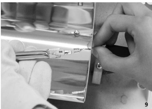
9. CONNECT THE MALE FASTONS OF THE NEW BULB TO THOSE OF THE TWO CORDS. COVER THEM WITH THE CAPS AND REPOSITION THE BULB IN THE SEAT OF THE TWO SPRING CLIPS. DO NOT TOUCH THE BULB WITH YOUR BARE HANDS.
